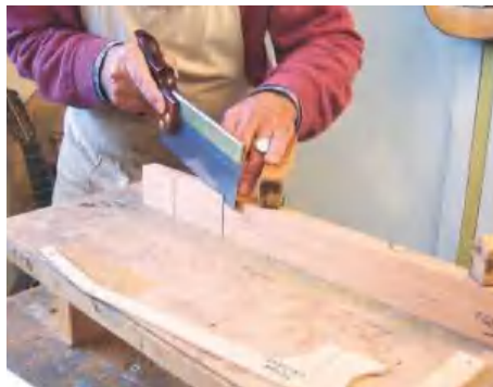
▲ Pic.14 Cutting the headstock scarf joint
